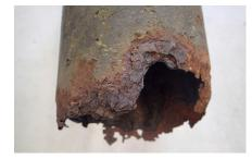
Corrosion damage at the base of the signal post
