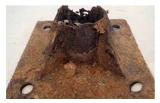
Corrosion damage of the baseplate
